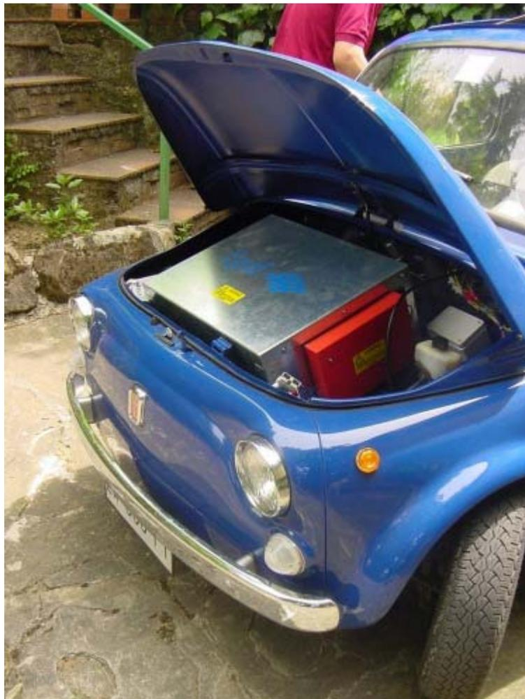
*Fig 4. The battery pack. These lithium polymer batteries contain as much energy as about one liter of gasoline. Nevertheless, the engine is so efficient that the car can run for 100 km, if driven gently.*
